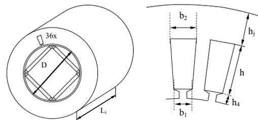
Fig 1. Machine dimensions and definition of optimisation problem arguments  $\{D, h\}$ .
