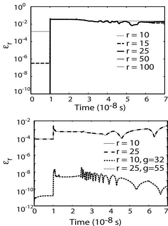
**Fig. 3.** Relative errors over all nodes for the reduced models created by TPWL (top) and by POD (down).
