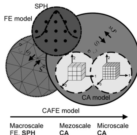
Fig. 1. Scheme of the data flow in the CAFE model.
