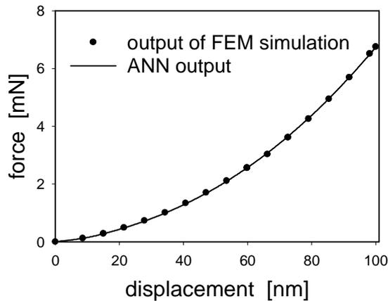
Fig. 1. Results of the network test set for work-hardening curve ( $n = 0.15$ ,  $E = 370$  GPa,  $K = 100$  MPa).
