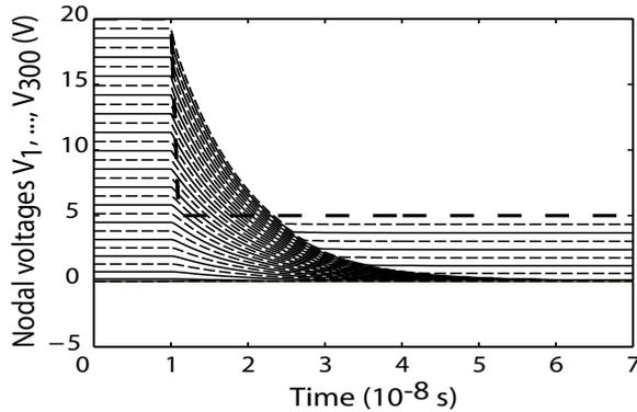
**Fig. 2.** Numerical solution of the full-scale nonlinear diode chain model.
