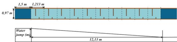
Fig. 1. Ground and plant for the fishway.
