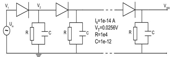
Fig. 1. Structure of the test circuit
