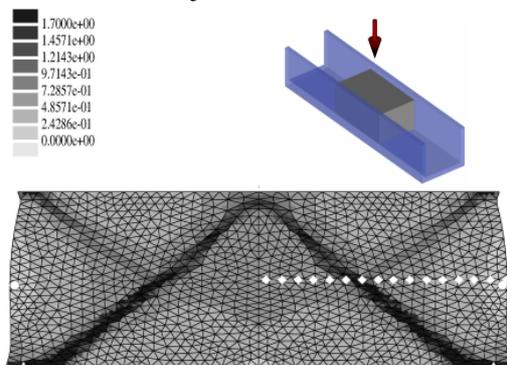
Fig. 2. View of the channel test (top) and cross section of the sample after compression showing distribution of strains and location of points, at which the hardness was measured.
