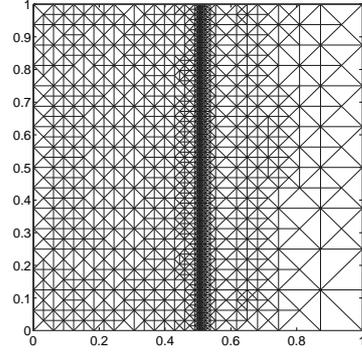
**Fig. 1.** Adaptive mesh obtained by steering the local refinement process via  $\eta$ .
