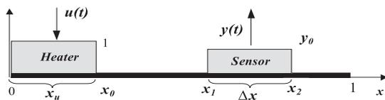
Figure 1. The one dimensional heat object.
