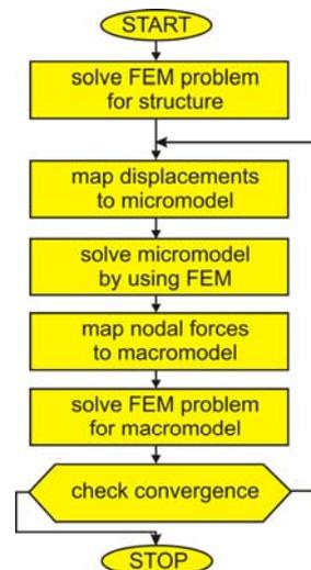
Fig. 2. Algorithm for macro-micro FEM
