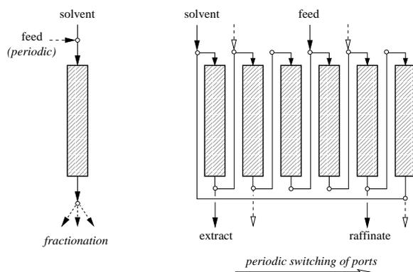
**Fig. 1.** Process schemes for discontinuous batch chromatography (left) and the continuous simulated moving bed (SMB) process (right).
