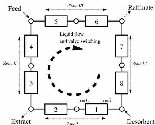
**Fig. 1.** Schematic diagram of standard SMB: 8 column type with two columns in each zone
