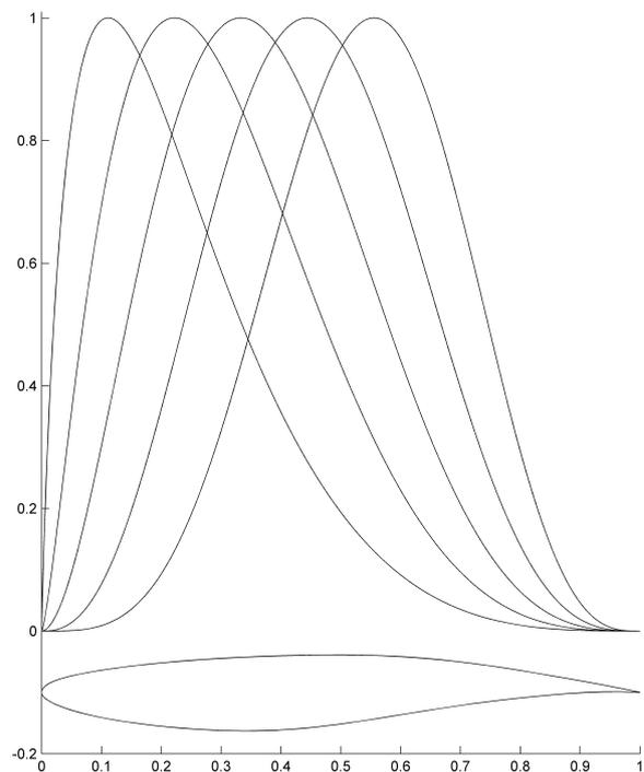
Fig. 1. Hicks-Henne parameterization with 5 basis functions
