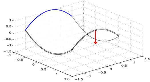
**Fig. 1.** Shell (hyperbolic paraboloid) with thickness  $t = 0.03$ , Dirichlet boundary conditions at  $x = -1$  and a downward force at  $x = 1, y = 0$
