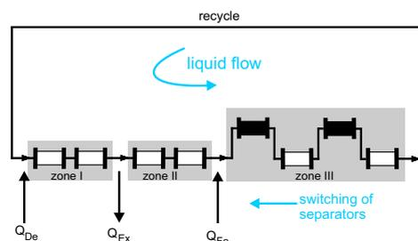
**Fig. 1.** Hashimoto three-zone configuration (reactors: black, separators: white)
