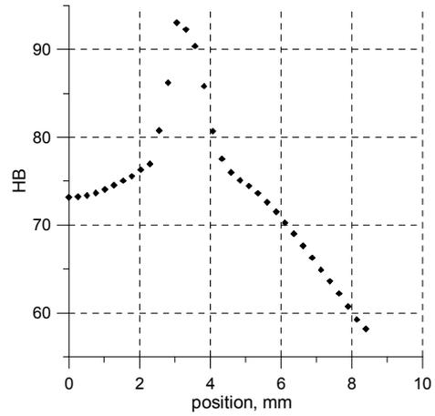
Fig. 3. Harness along the sample, which is used as an input for the inverse analysis.
