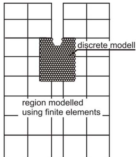
Fig. 1. A two-scale model of the material system
