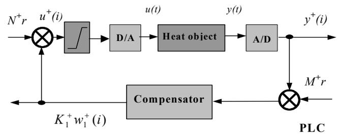
Figure 2. The closed-loop control system with dynamic discrete compensator.
