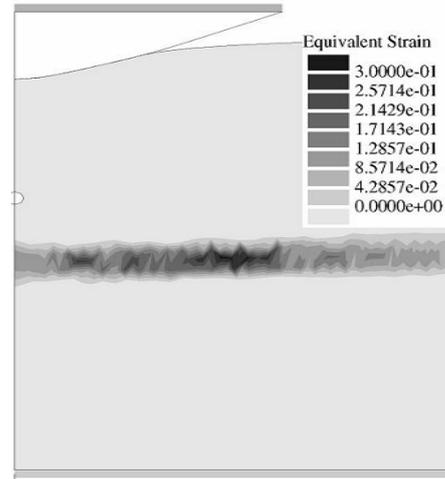
Fig. 3. Strain distribution in the 2D axisymmetric sample for material parameters determined from the inverse analysis for the case I.
