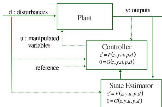
**Fig. 1.** Block Diagram of Model-Based Control Structures
